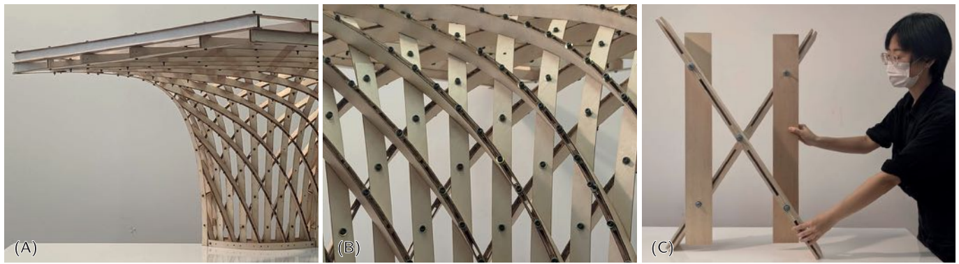
Fig. 18. A timber prototype was constructed at 1:5 scale (80 x 80 cm). The combination of double asymptotics and interwoven geodesics create a strong web, halves the buckling length and braces the structure. A 1:1 joint was built to test the laminated joints, and bolt connections.
