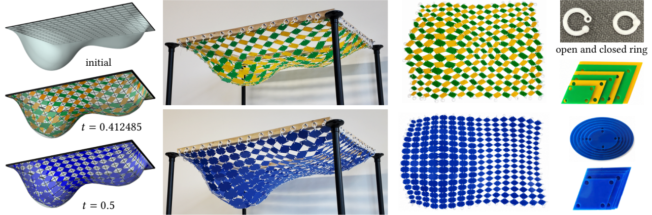
Fig. 1. A freeform surface with planar rectangular boundaries is tiled by an isogonal quad mesh composed of similar parallelograms in a checkerboard pattern. Two similar layouts are obtained under two prescribed control ratios. At the computed ratio t = 0.412485 , the upper layout features yellow and green parallelograms with identical interior and diagonal angles arranged in mirrored similarity. At t = 0.5 , the lower layout adopts a half-and-half pattern, where the entire structure is formed by similar rhombuses, half of which are replaced by their area-minimizing circumscribed ellipses. Physical prototypes show good agreement with numerical results. The similarity of laser-cut acrylic panels (parallelograms, rhombuses, and ellipses) is clearly observable in the top view.
